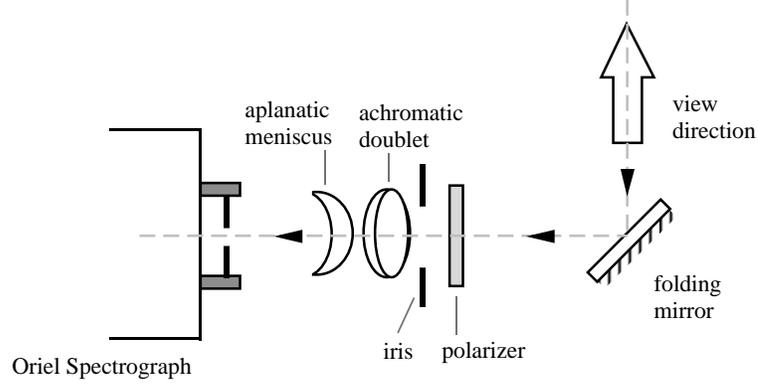
Figure 6.1: Schematic of the detector's focusing optics.
