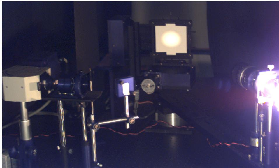
Figure 2.5: The gonioreflectometer with its detector optics (left) and light source optics (right) exposed. A white Spectralon sample (middle) is shown illuminated by the source at  $\theta_i = 45^\circ$ . The detector is viewing the sample via the folding mirror at  $\theta_r = 0^\circ$ .
