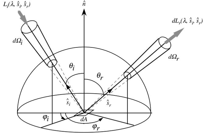
Figure 1.1: Reflection geometry showing cones of incident and reflected light above a surface element.
