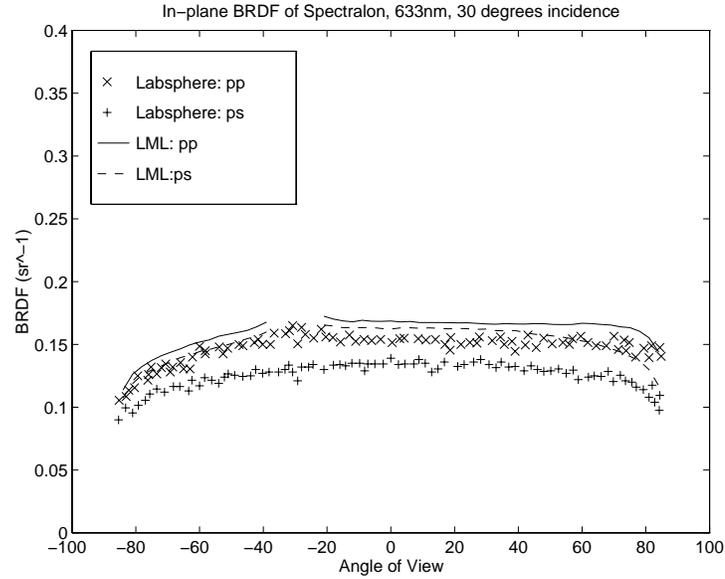
Figure 9.6: BRDF of Spectralon on the incidence plane at  $\theta_i = 30^\circ$  for incidence source of  $p$  polarization, 633nm wavelength. The reflection is measured for both  $s$  and  $p$  polarizations. Data published by Labsphere in [27], and measurement made by our gonioreflectometer (LML) are plotted for comparison purposes.
