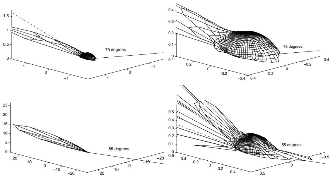
Figure 9.9: BRDF of latex blue paint at a 450nm wavelength, at incidence angles of  $75^\circ$  and  $85^\circ$ . The figures on the right are magnifications of figures on the left. The radius from the origin corresponds to the BRDF value. Both the incidence direction (solid line) and the reflection direction (dashed line) lie on the incidence plane.
