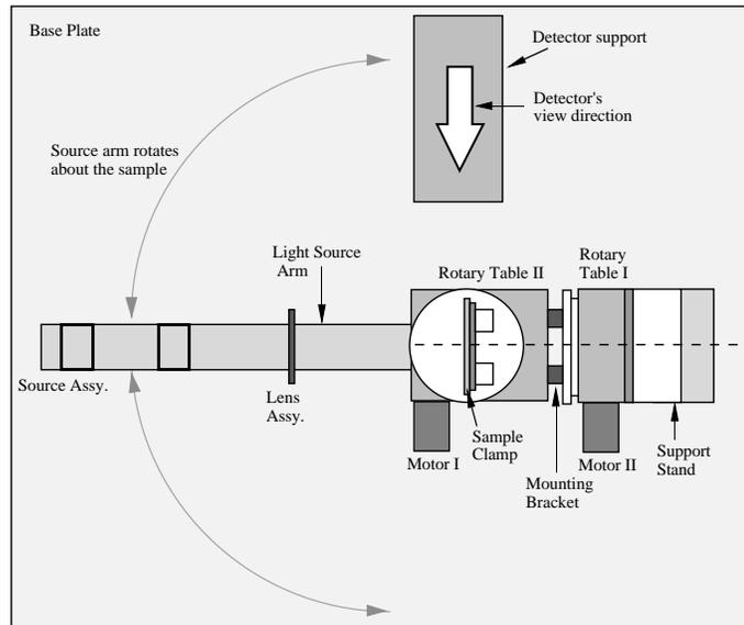
Figure 2.2: Bird's eye view of the original Kodak Goniometer.
