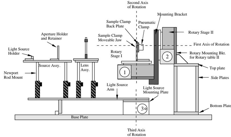
Figure 2.1: Side view of the original Kodak Gonioreflectometer.
