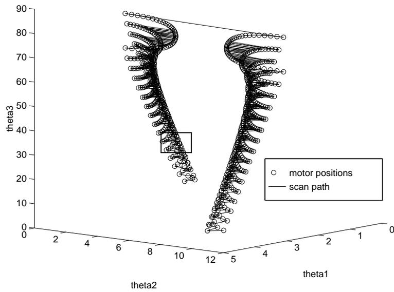
Figure 3.5: Optimized scan path, in solid line, shows the sequence to scan all the pre-determined measurement positions in  $\theta_1$ ,  $\theta_2$ , and  $\theta_3$ . The three axes are scaled by the individual speeds of the motors to show the travel-time difference among the positions.
