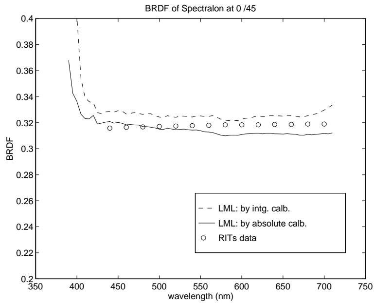
Figure 9.5: Measured BRDF (unpolarized) of Spectralon with source incident at  $\theta_r = 0^\circ$ ,  $\varphi_r = 0^\circ$ , and view direction at  $\theta_r = 45^\circ$ ,  $\varphi_r = 180^\circ$ . BRDF calculated by absolute calibration (abs.) and diffuse reference calibration (intg.) are shown. Measured data published by RIT are plotted in circles.
