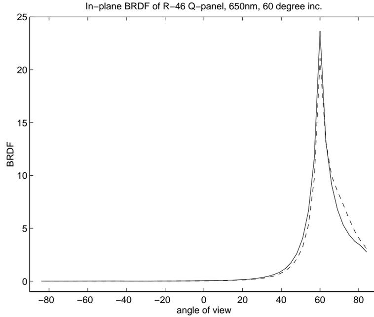
Figure 9.13: BRDF of the Q-Panel R-46, a matte-finished stainless steel, measured in two crossed incidence planes, at  $\theta_i = 60^\circ$  and wavelength = 650nm. The two curves are on two crossed incidence planes, one (-) parallel, and the other (- -) perpendicular to the machining direction. The discrepancies indicates the anisotropy of the material.
