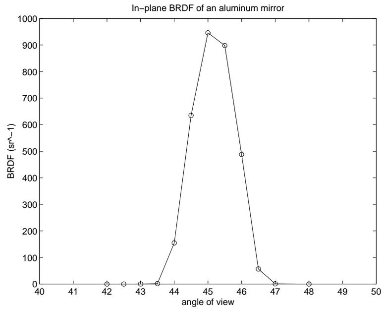
Figure 9.2: Measured BRDF of a vacuum coated aluminum mirror on the incidence plane, at incidence angle of  $45^\circ$  and at wavelength of 550nm. The specular reflection of the mirror is equal to the product of the peak BRDF value, the value of the detector solid angle, and  $\cos 45^\circ$
