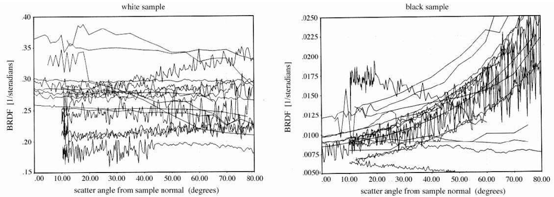
Figure 1.2: BRDF measurements of white (left) and black (right) samples, at 633nm wavelength, by eighteen facilities. The specular direction is at  $10^\circ$ . The white sample has a flat BRDF and the black sample shows increasing reflectance at large angles. [From page 234, [18].]
