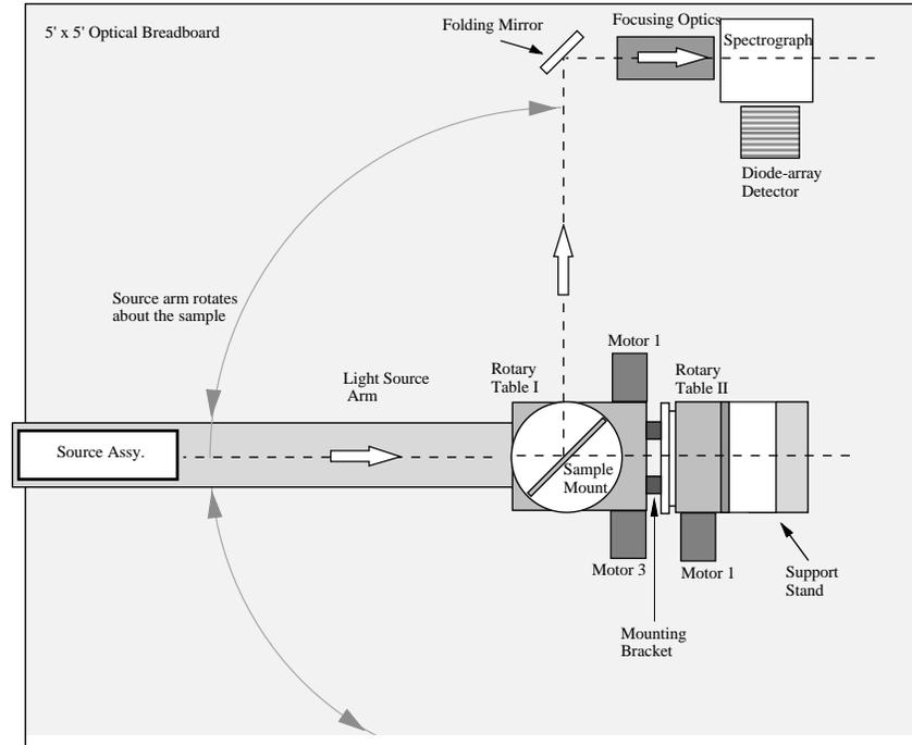
Figure 2.3: Bird's eye view of the modified Gonioreflectometer. The white arrows indicate the direction of illumination and reflection.
