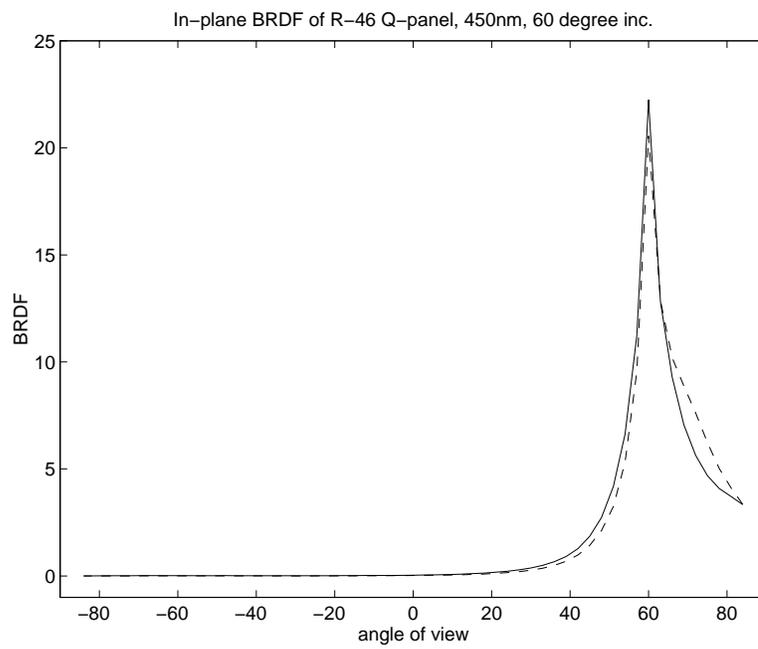
Figure 9.14: BRDF of Q-Panel R-46, a matte-finished stainless steel, measured in two crossed incidence planes at an incidence angle of  $60^\circ$ . The plots are similar to those in Figure 9.13, but with wavelength at 450nm.
