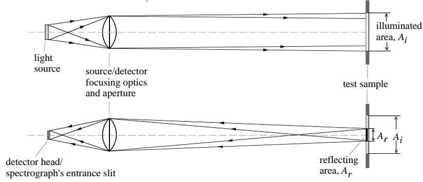
Figure 4.3: Optical configurations of illumination and radiance detection.
