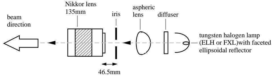
Figure 5.1: Schematic of the light source assembly.
