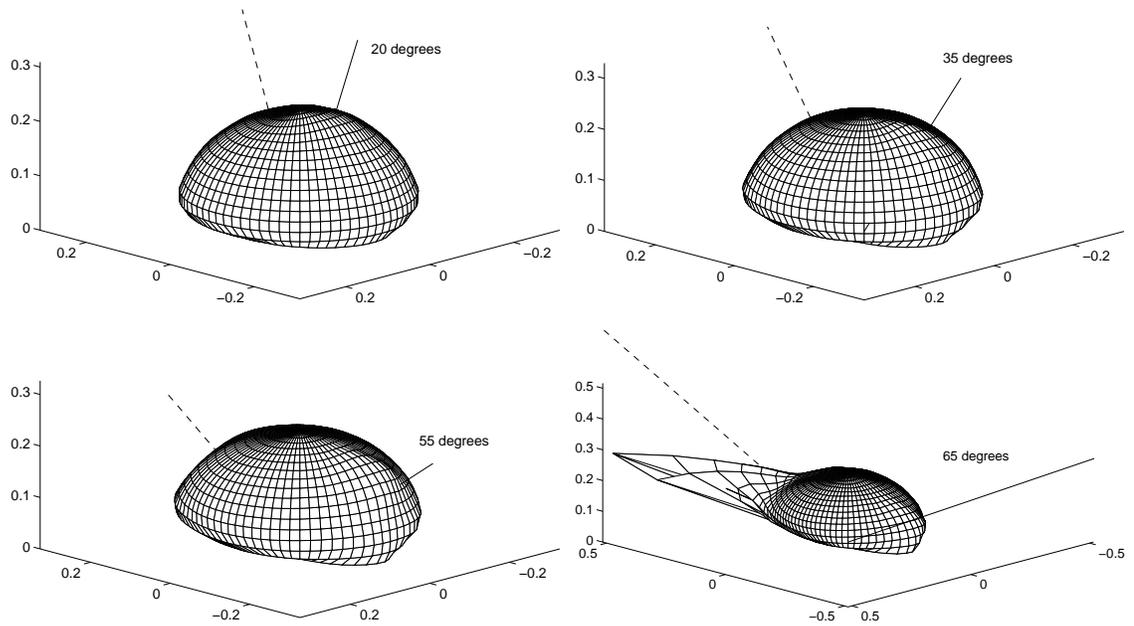
Figure 9.8: BRDF of latex blue paint at a 450nm wavelength at incidence angles of  $20^\circ$ ,  $35^\circ$ ,  $55^\circ$ , and  $65^\circ$ . The axes are in true BRDF units. The radius from the origin corresponds to the BRDF value. Both the incidence direction (solid line) and the reflection direction (dashed line) lie on the incidence plane.
