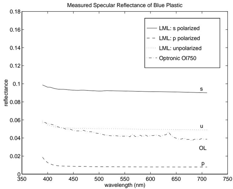
Figure 9.4: Comparison of polarized specular reflection of a blue plastic at an incidence angle of  $45^\circ$ , measured with the Optronic OL740-75M specular reflectometer and our gonireflectometer. The measurement made by the Optronic OL740-75M has not been adjusted for polarization bias.
