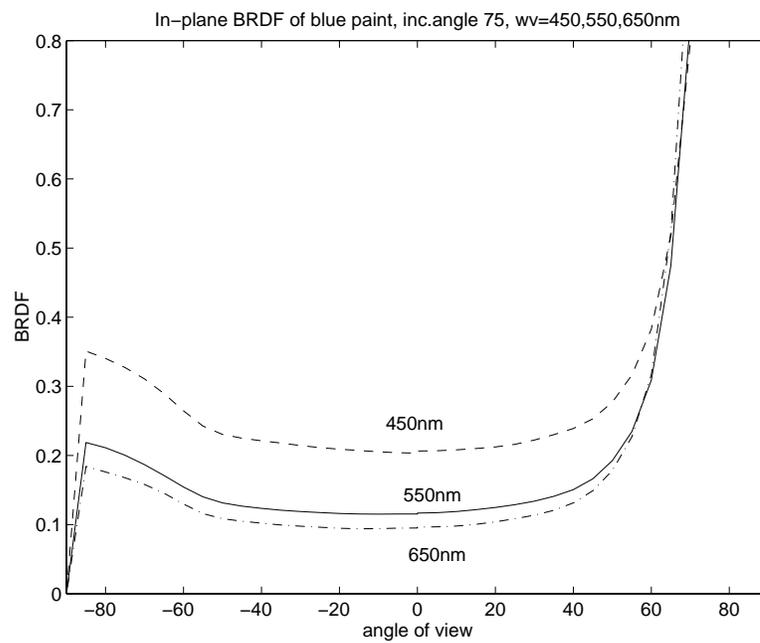
Figure 9.11: Measured BRDF of the blue paint on the incidence plane at  $\theta_i = 75^\circ$ , and  $\lambda = 450, 550, 650\text{nm}$ . The forward scattering increases as wavelength increases but the diffuse part is dominated by the “color” of the paint.
