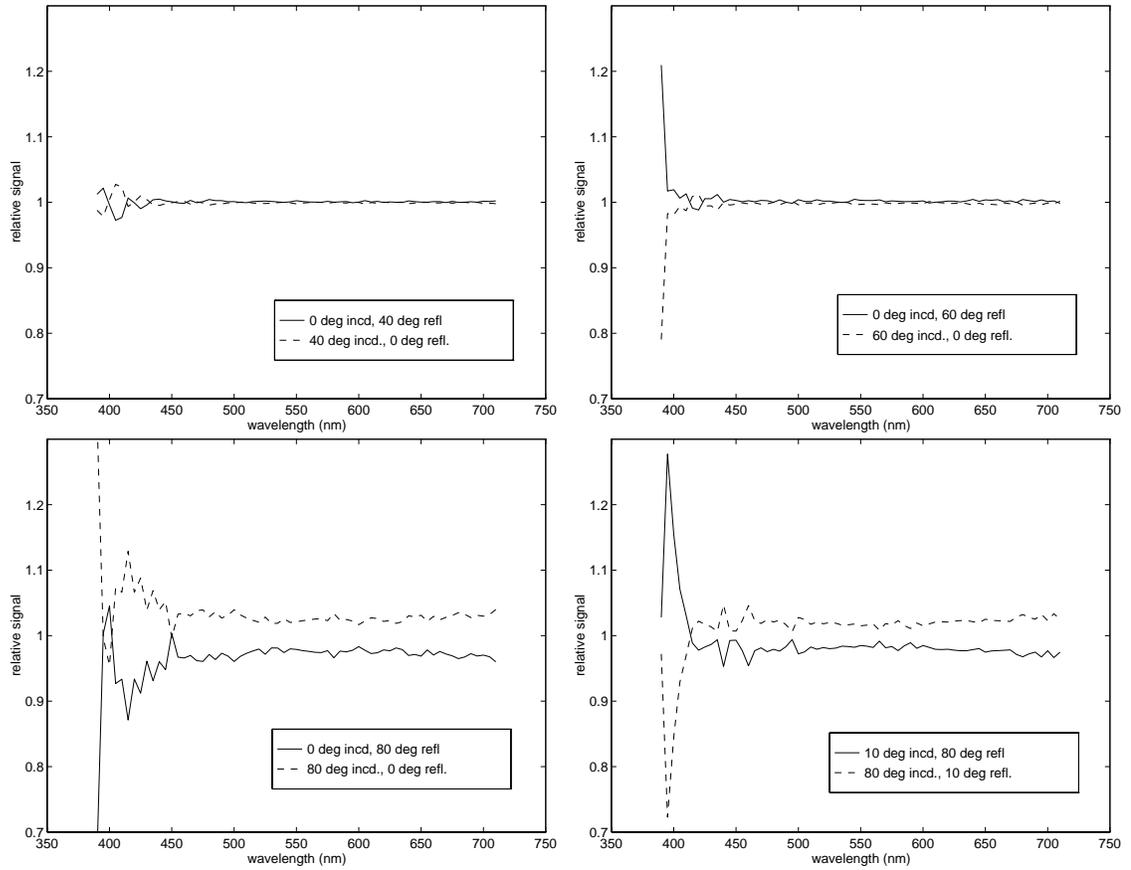
Figure E.1: Reciprocal measurements made of Spectralon sample at various source-view directions. The wavelength is  $\lambda = 550\text{nm}$ . Each curve is normalized by the average of the two curves. A perfect reciprocal pair of measurements would have values at 1.
