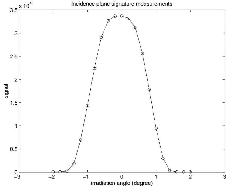
Figure 9.1: The signature is measured (at  $\lambda = 650\text{nm}$ ) with the light source moving from  $\theta_3 = 178^\circ$  to  $182^\circ$ , without a test sample. The broadened curve shows the effect of aperture convolution since the detector has a finite aperture and the reflecting area on the sample plane is finite.
