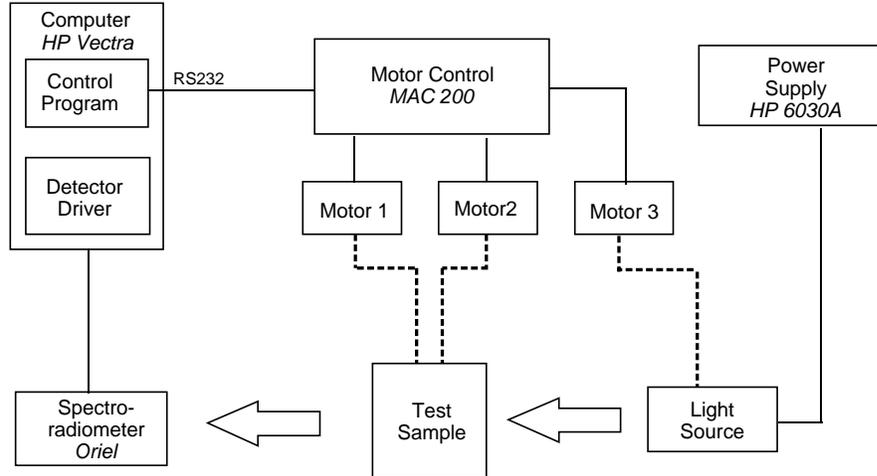
Figure 2.4: Block diagram showing the schematic of the measurement system.
