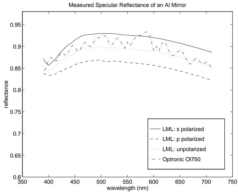
Figure 9.3: Comparison of polarized specular reflectance of a vacuum-coated aluminum mirror at an incidence angle of  $45^\circ$ , measured with the Optronic OL740-75M specular reflectometer and our gonireflectometer. The unpolarized measurement is the average of the  $s$  and  $p$  measurements. Measurement made by the Optronic OL740-75M has not been adjusted for polarization bias.
