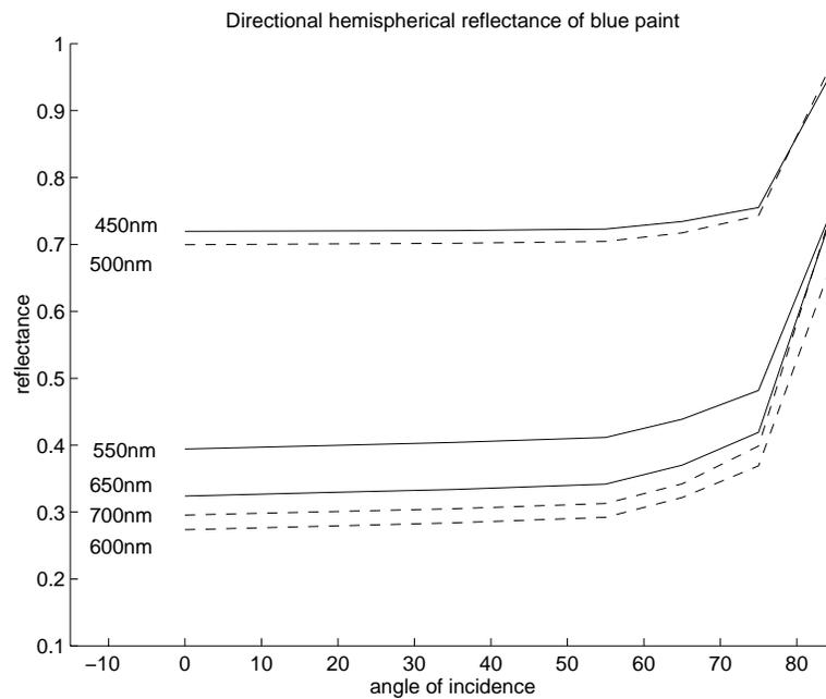
Figure 9.15: Directional-hemispherical reflectance of the latex blue paint, plotted for various wavelengths as a function of incidence angle. The incidence angles where measurements were made are  $0^\circ$ ,  $20^\circ$ ,  $35^\circ$ ,  $55^\circ$ ,  $65^\circ$ ,  $75^\circ$ , and  $85^\circ$ . The reflectances are computed by integrating the BRDF over the entire hemisphere.
