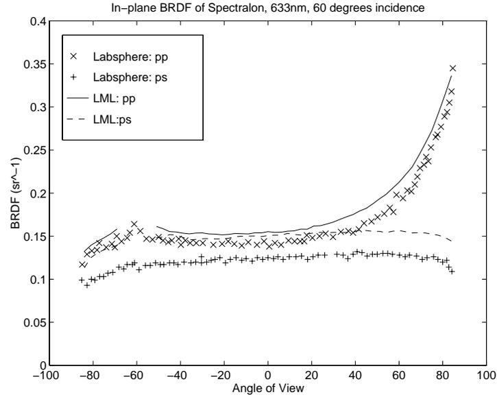
Figure 9.7: BRDF of Spectralon on the incidence plane at  $\theta_i = 60^\circ$  for an incidence source of  $p$  polarization, 633nm wavelength. The reflection is measured for both  $s$  and  $p$  polarizations. Data published by Labsphere in [27] and measurements made by our gonioreflectometer (LML) are plotted. The measurements agree well.
