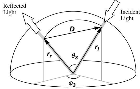
Figure 3.3:  $\theta_3$  is uniquely defined by the incidence and reflection direction.
